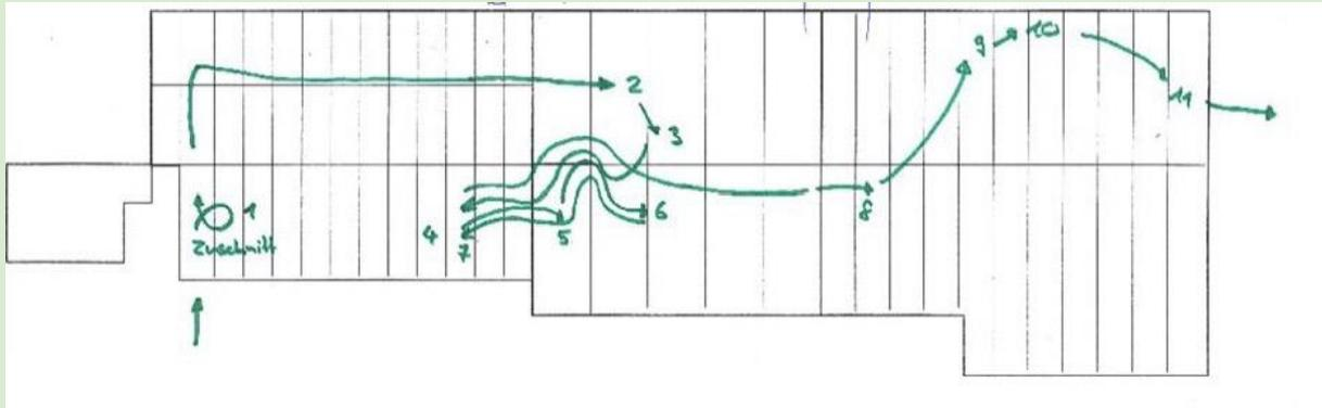
Figure 5.10: Schematic representation of the routes for the operations needed to manufacture fronts
