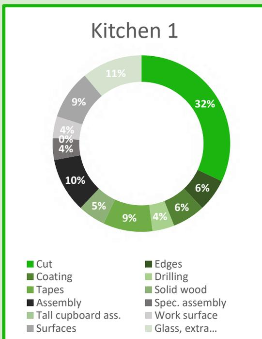
Figure 5.5: Proportional amount of time needed for each manufacturing step (kitchen 1)
