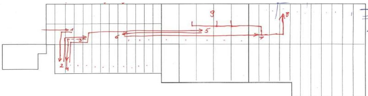
Figure 5.11: Schematic representation of the routes for the operations needed to manufacture cabinets
