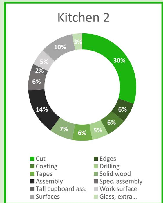
Figure 5.6: Proportional amount of time needed for each manufacturing step (kitchen 2)
