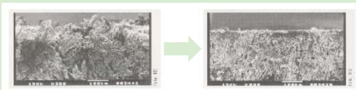
Figure 5.18: Microscopic images of a milled medium-density fiberboard, unsmoothed (left) and thermally smoothed (right)
